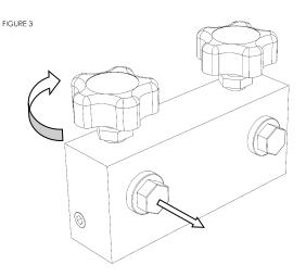
Adjusting the knob on Needle Valve 2 will control the rate at which hydraulic fluid exits Outlet Port
