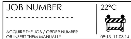
In the JOB NUMBER page, the user can insert the current job code (max 16 digits) either by reading a barcode (symbology Code 128), or inserting it manually.
