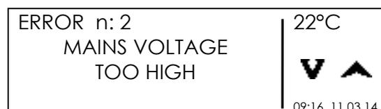
**Check the voltage stability and the power capacity of the generator before starting the welding.**
