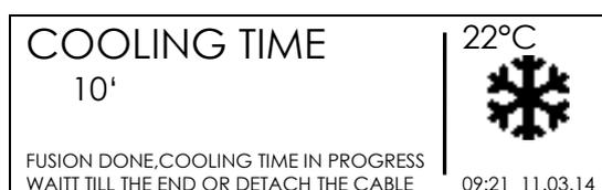
After the completion of the fusion process, the protocol summary and the remaining cooling time, if contained in the barcode, are displayed alternately. Messages are active till the user will press the STOP/ESC (O) button or will detach the fusion cables from the fitting, to proceed with the next welding.
