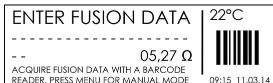
The user has two ways of inserting the fusion parameter using the barcode information:
