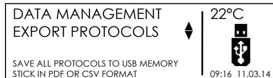
Insert the USB memory stick on the USB connector available on the rear panel of the machine, then select EXPORT PROTOCOLS. Using the buttons (▲)(▼) scroll the menu and choose the export type:
