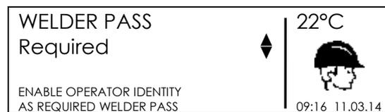
Select by (▲)(▼) the identification mode and press START/OK ( I ) to confirm the setting. To cancel the operation press STOP/ESC ( O ).
