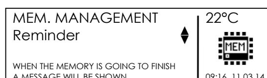
Select by (▲)(▼) the mode and press START/OK ( I ) to confirm the setting. To cancel the operation press STOP/ESC ( O ).
