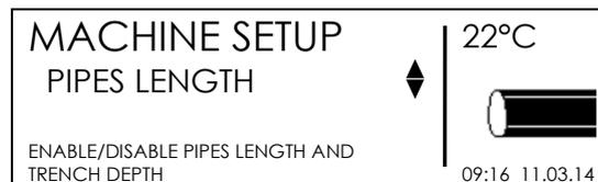
Select by (▲)(▼) buttons if You want to enable or disable the functionality and push START/OK (I) to confirm the setting.
