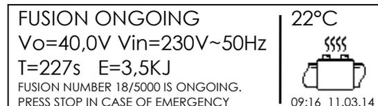
During the fusion process, the display shows the information concerning the output voltage, the input voltage and frequency, the remaining fusion time and the applied energy.
