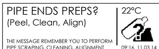
If FUSION PREPARATION alert is activated, the display shows a message which requires confirming the pipes preparation (scraping, cleaning, and alignment) has been done. If it has been executed, press START/OK (I) to proceed.
