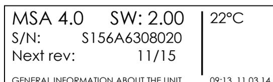
Connect the machine to the power mains or generator, already started, and switch on the machine. The display shows the machine information (machine type, serial number, software version and date of the next revision).
