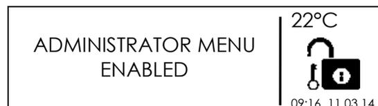
the complete menu set (both for DATA RETRIEVAL and MACHINE SETUP) is available. Then the machine responsible can change the configuration to suit his needs, as described in the **Configuration Settings** and in the **Data Management** chapters of the Operating Manual.
