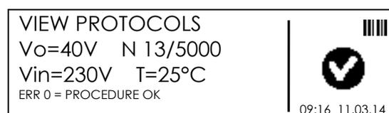
The buttons (▲)(▼) allow to scroll up and down the list of protocols. Pressing STOP/ESC (O) the user can go back to DATA RETRIEVAL menu again.
