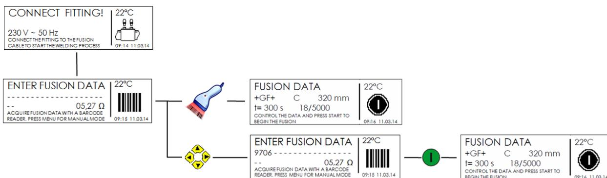
As soon as the data are correctly read, the machine will compare the measured fitting resistance with the nominal value written into the barcode. In case they match, the electro-fusion unit will confirm with a beep and show on the display a summary of the captured fusion parameters: fitting details and time of the welding process.
