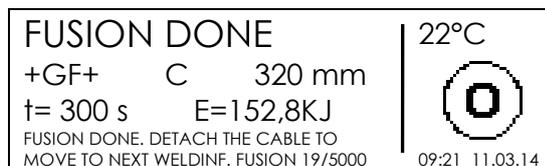
As soon as the fusion process is correctly ended the display shows briefly the information concerning the real fusion time and the total energy applied to the jointing. These data will be part of the welding protocol stored into the internal memory.
