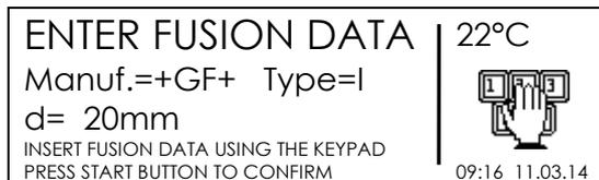
When the insertion is finished, press START/OK (I) to move forward to the fusion process.
