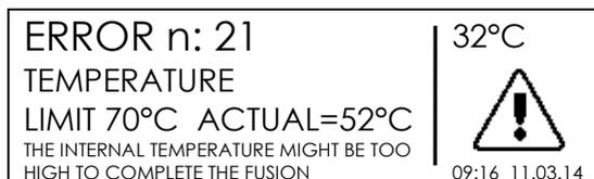
The message above is an advice, to inform the user the fusion process may not be concluded successfully due to internal temperature of the machine. Since the fittings have different curves depending on manufacturer, size, technology parameters, it does not prevent the user for going forward, if he is sure, based on his experience, the fitting can be welded.
