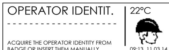
In the OPERATOR IDENTITY page, the user can insert the operator code by reading the barcode printed out in the welder pass, or by inserting the name manually.
