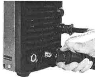
Installing torch cable
