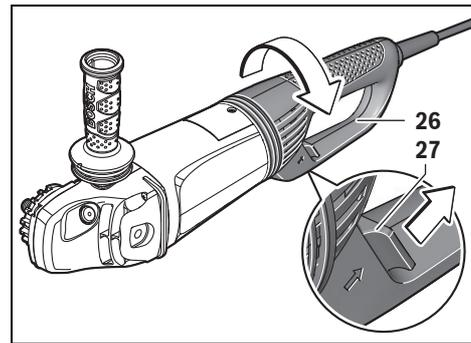
The main handle **26** can be rotated with respect to the machine housing toward the left or right in steps of  $90^\circ$ . In this manner, the On/Off switch can be brought into a more convenient position for special working situations, e.g., for cutting operations using the cutting guide with dust extraction protection guard **22** or for left-handed persons.
