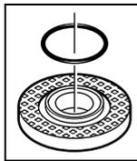
A plastic part (O-ring) is fitted around the centring collar of mounting flange **10**. **If the O-ring is missing or damaged**, the mounting flange **10** must be replaced before resuming operation.
