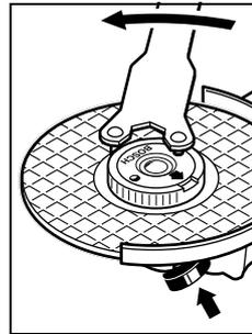
A properly attached, undamaged quick-clamping nut can be loosened by hand when turning the knurled ring in anticlockwise direction.
