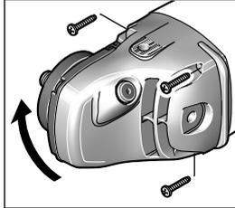
The machine head can be rotated with respect to the machine housing in 90° steps. In this manner, the On/Off switch can be brought into a more convenient position for special working situations, e. g., for cutting operations using the cutting guide with dust extrac-
