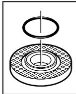
A plastic part (O-ring) is fitted around the centring collar of mounting flange **7**. **If the O-ring is missing or damaged, the mounting flange 7 must be replaced before resuming operation.**
