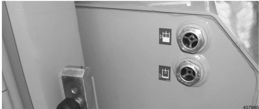
Fig. 39 Schild MIN/MAX Hydrauliktank
