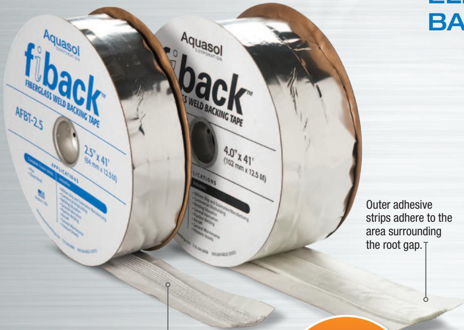
Woven fiberglass strip is applied to the back of the weld to eliminate or reduce the need for back purging and create a weld pool enclosure.
