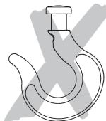
Never attach the load to the tip of the hook. The lifting tackle must always be seated in the saddle of the hook.
