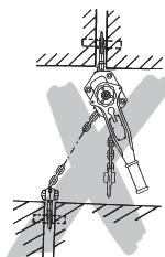
The load chain must not be used as a chain sling.
