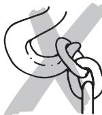
Do not use the chain stop as an operational limit device.
