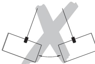
The load must not be moved into areas which are not visible to the operator. If necessary, he must ensure he is given help.
