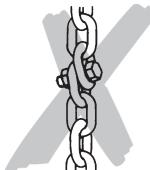
Removing the safety latches from top and/or load hooks is forbidden.
