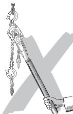
The unit must never be operated with more than the power of a person.
