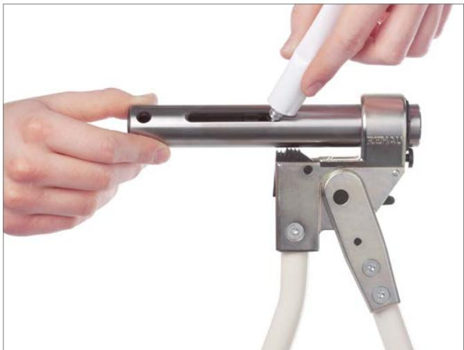
Grease the inside of the cylinder regularly (tube of lubricant is enclosed); ensure the outer surface of the cylinder remains dry. Compression jaws are not greased.
