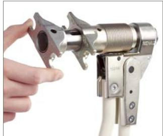
3. Secure both jaws into place by fully inserting the short locking pin into the long compression jaw and the longer locking pin into the shorter jaw.
