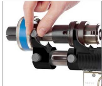
Before using the tool, check to make sure the seating is completely in the clamping jaw and clamping action of the expanding device in the clamping jaw are correct (i.e. to avoid falling out).
