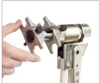
4. Always change the compression jaws in the starting position (tool handle in maximum configuration).
