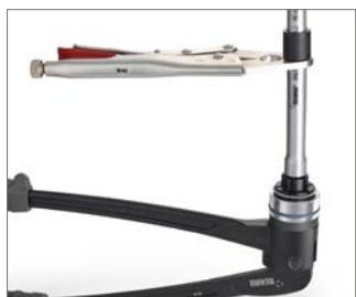
2. By rotating the tool cylinder, the compression jaws can be brought into the correct working position.
